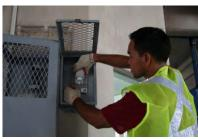
The diffusive sampler can be used for measurements of a variety of air pollutants. In this project only  $NO_2$  was measured.
