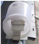
The technique is based on the concept of diffusion. In diffusive sampling the gas is transported by turbulent diffusion through the open end into the absorbent where the gas is absorbed by the sampling medium through molecular diffusion.
