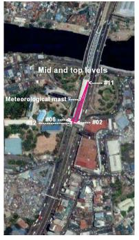
The numbers and colors indicate the various locations and "lines" along which the monitoring was accomplished. The yellow line is the "background" area (#16, #17, and #18) around 250 meters south of the MRT station and the photocatalytic painted areas. Also #01 and #10 are background locations painted with ordinary paint.
